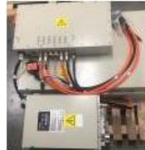
Figure 8-3 Orange High Voltage Connection Line
